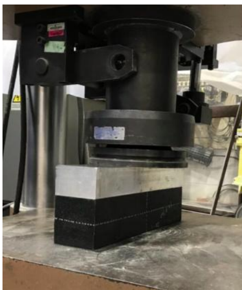
Figure 10: Representative failure test view: Steel holder rigid bar.
