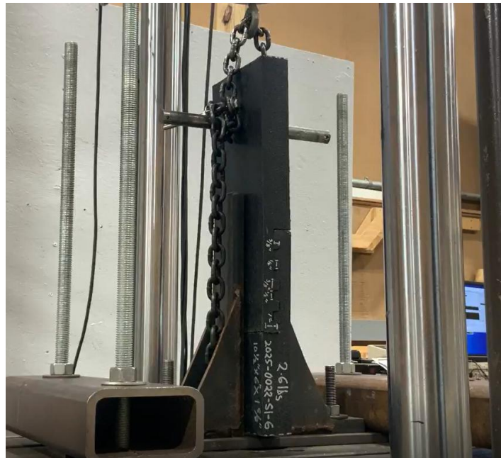
Figure 17: Representative shear strength test view: Constrained Condition.
