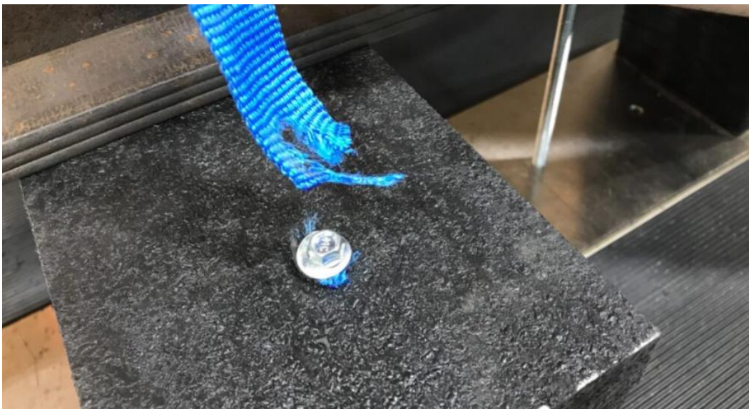
Figure 13: Representative picture of the failure mode in the Steel Holder.
