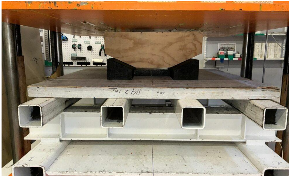
Figure 5: Representative compression test view: Steel holder adjustable pallet assembly.
