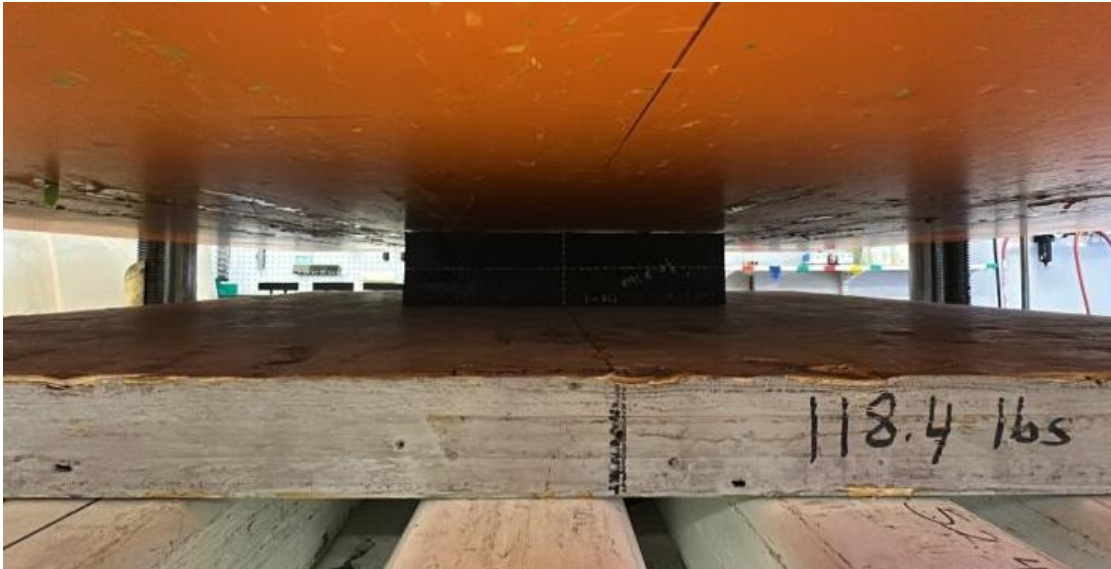
Figure 8: Representative compression test view: Steel holder rigid beam.
