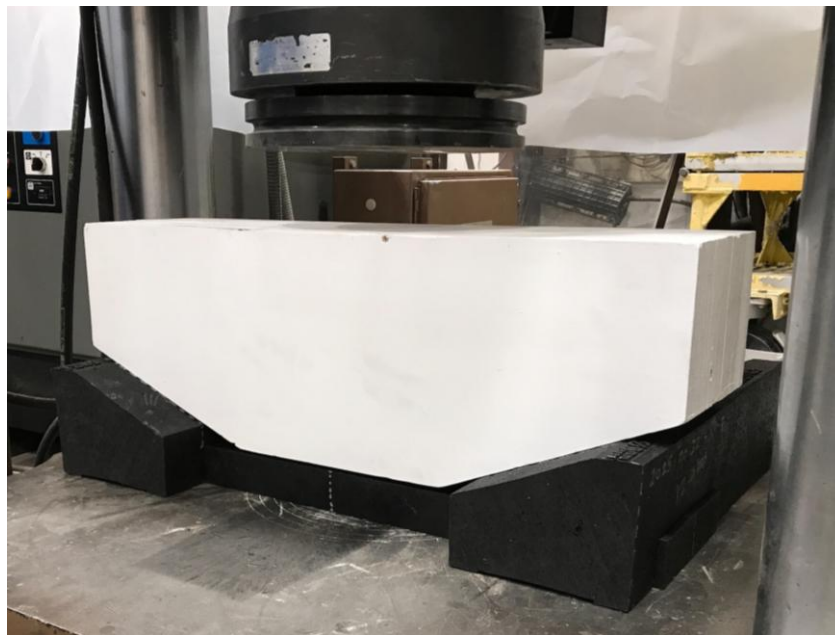
Figure 7: Representative fail test view: Steel holder adjustable pallet assembly.
